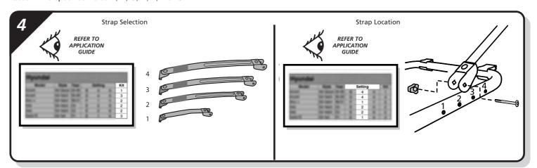
Refer to the enclosed application list to find the correct metal strap for your car. Refer to the enclosed application list to find the correct clamp bolt hole for your car. Insert the bolts, from the outer faces,
